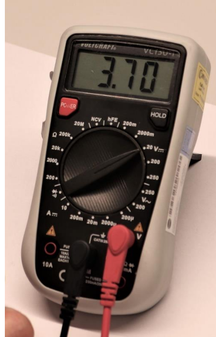
Figure 12: Settings at the multimeter for voltage measuring as an example image
