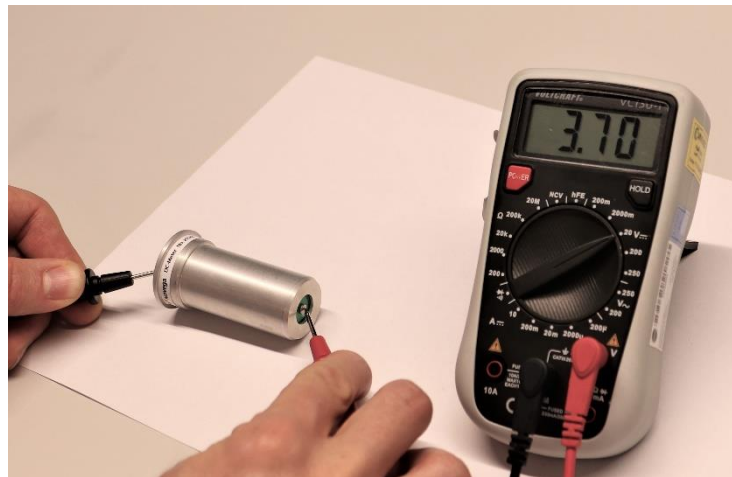
Figure 13: Measuring the battery voltage of the DC-Meter as an example image
