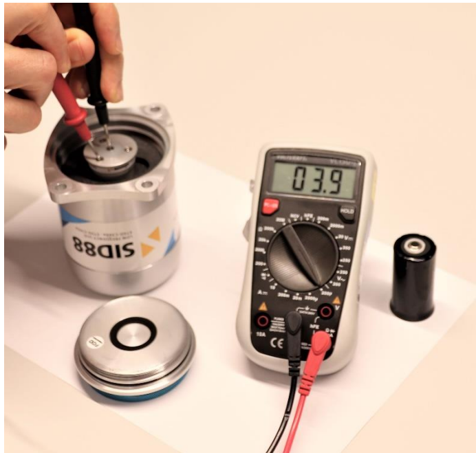
Figure 11: Connecting the DC-Meter with the Multimeter as an example image
