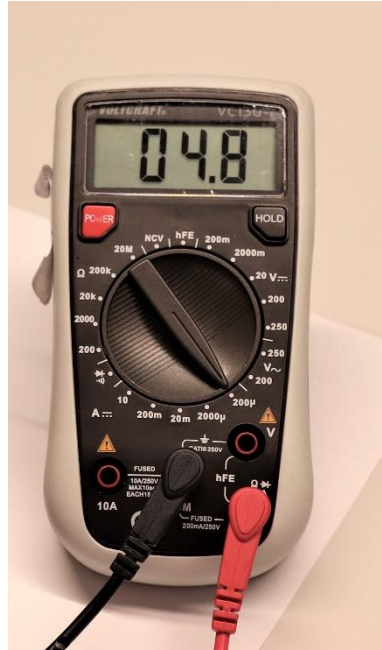
Figure 6: Settings at the multimeter for current measuring as an example image
